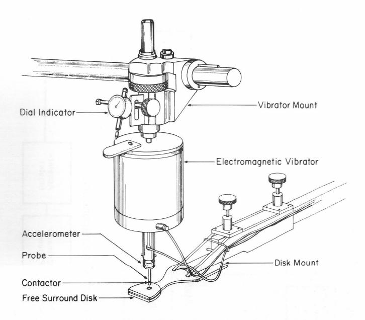
Figure 2. A Graphic Representation of the Vibrator Assembly Portion of the Instrumentation
